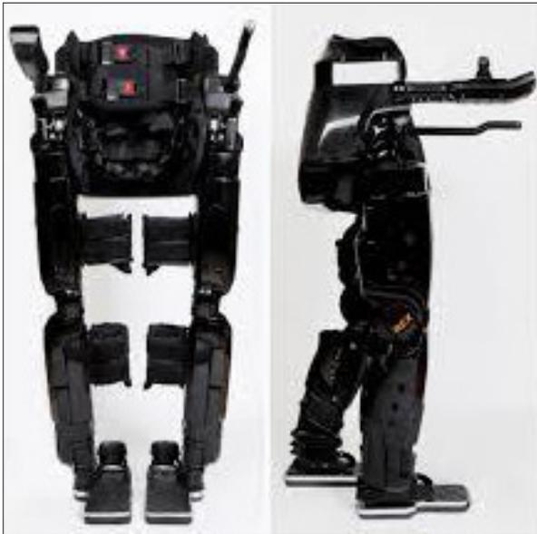
Fig. 1. Rex Bionics exoskeleton [5].
